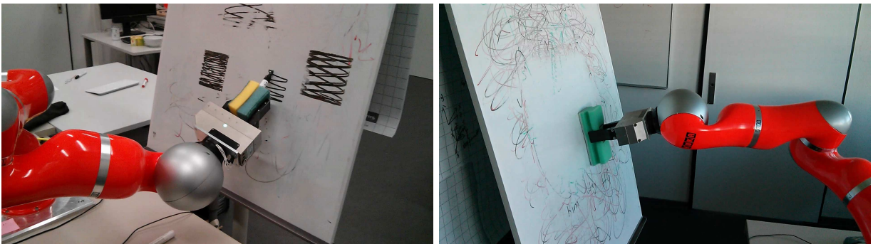
Fig. 3. Compliant drawing (left) and whiteboard wiping (right) using a KUKA LWR arm. The exact pose of the whiteboard is unknown and the robot has to adjust its motions using joint feedback. During drawing (left), an additional low-priority goal is attached to the arm, which can be used to prevent the arm from blocking the view; however, if necessary for fulfilling the high-priority end effector goal, the low priority goal can be violated. Disabling compliance during wiping either directly leads to loss of contact or causes the robot to push the whiteboard away and to then lose contact. Disabling compliance during drawing leads to excessive force on the pen as well as frequent loss of contact and large gaps in the drawing. If compliance is disabled from the beginning, the robot is unable to find the correct distance at all. If compliance is enabled, the whiteboard can also be moved during execution and the robot adjusts its motions accordingly.
